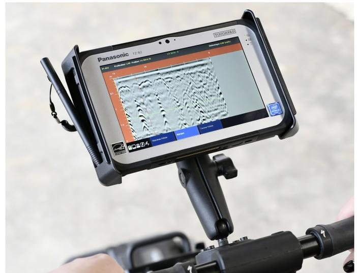
The Georadar detection operation consists in moving perpendicularly to the pipe sought (which supposes having an approximate idea of where it is) and then identifying on a radargram - which can be consulted live from the device's screen - the top of a hyperbola that represents the upper generator of the pipe sought.
